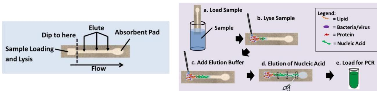
Figure 1. Left: patterned cellulose channel using modified lithography. Elution regions are equally spaced. Right: overall sample preparation process: (a) load sample on paper; (b) add TE lysis buffer and incubate for 5 minutes; (c) add TE elution buffer; (d) elute nucleic acid for PCR from three regions by cutting the paper; (e) load nucleic acid in pre-mixed solution of PCR reaction. The flow shows theoretical separation of various components within paper.
